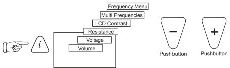
When the "i" (information) pushbutton is pressed, the display will show the volume level of the audio; use the "+" and "-" pushbuttons to increase/reduce the volume or turn the beeper off (off low - medium - high).
