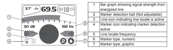
Note that both icons are now illuminated indicating that dual configuration is activated. Energize the cable with 512 Hz, 640 Hz or 8.192 kHz as instructed in the vLoc user handbook. Select the antenna configuration by using the "M" pushbutton. Note that the left/right arrows indicate the cable position and **not** the marker position.
