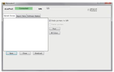
Connect the vLoc Receiver to the PC using a USB to Mini USB cable. The PC should recognize the vLoc and the display will now change to the below or similar.
