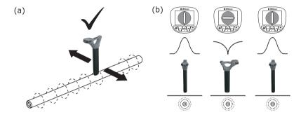
The receiver should be kept parallel to the ground – and should not be flipped up at the end of each pass. See diagram (a).
