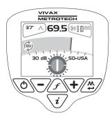
Re-trace your line back to a point where a solid signal direction is obtained. Precisely pinpoint the line and stand with your back to the direction of the transmitter as you did when you initiated the original sync, and press the "i" pushbutton then the enter/return pushbutton to re-sync with the transmitter signal.
