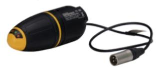
The LPC separation filter (LPC) is used to safely inject a trace tone to a live cable via a domestic mains socket, so that the cable can be traced from the premises to the connection in the street. It is suitable for connecting to voltages between 100V AC and 250V AC.
