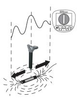
The vLocPro2 receiver must be used in a different orientation when locating a Sonde - due to the way the signal from the Sonde radiates. With the front of the receiver pointing across suspected direction of the Sonde - pinpoint forward and backward (across the Sonde) and then move along the line of the Sonde until the maximum peak is located (in other words rotate the receiver 90 degrees from the orientation normally used when locating pipes and cables).
