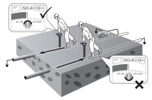
At some point you may find that the top or bottom portion of the compass (line direction indicator) bezel together with the SD icon and start flashing – this is indicating that synchronization with the transmitter has deteriorated and a reset is required.
