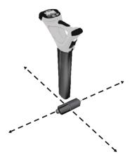
When over the peak position, the depth is automatically displayed. Press the "i" pushbutton to get a more precise depth reading.
