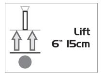
5. Raise the locator 6" (15cm) and again press the "i" button. The depth estimation will be displayed similar as shown below:
