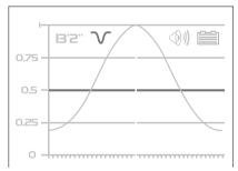
Now slowly move the locator to the side until the line on the graph reaches the 50% line. (or 70% if the 70% rule is used). At this point an audible beep will confirm this position is reached. Mark the ground at this point and then slowly return to the peak position. Continue past this position until the 50% mark is reached on the other side. Mark this position.
