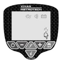
Press the "M" button as indicated by the hand. The screen will then revert to the one below with the front half of the circle red. This indicates that the reset was successful.
