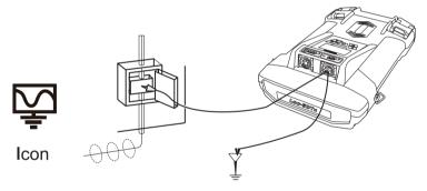
Wherever a direct connection can be safely made without the risk of injury, damage to customer's plant, or the transmitter, it is the best way of applying the transmitter's signal.
