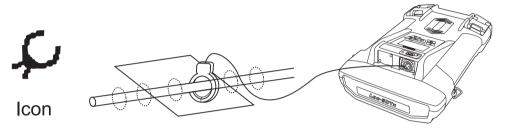
The clamp again is a precise way to apply the locating signal. It is generally used when access to the conductor cannot be achieved to make a direct connection (but there is sufficient access to place the clamp around the cable), or when it is not safe to make a direct connection because the target cable is carrying electricity.
