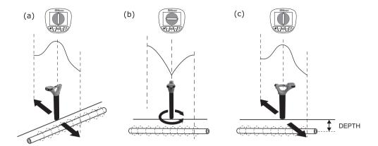
Once the position and direction of the cable has been established, stand with the base of the locator on the ground - with the locator in the absolute "Peak" position (over and in line). Then press the "i" information pushbutton briefly, the current and depth will be displayed.
