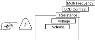
2. Use the "+" and "-" pushbuttons to scroll through the available frequencies, and bring the wanted one in the first box.
